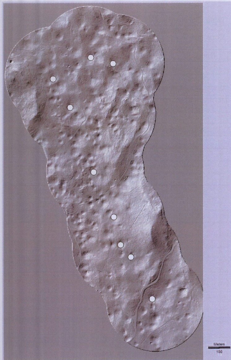
Figure 24: Trnovo test site. The shaded image of the high resolution (1 meter) lidar digital terrain model. White dots indicate the locations of the nine treatment plots within this test area. An accurate high-resolution DTM is needed as a precondition for many lidar based forest stand analyses, because we first need to know the relative height of each point above bare ground. This height is computed as the difference between the point elevation and the local DTM elevation.
