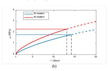
Figure 2: Time development of the stress in the concrete ring,  $\sigma$ , determined by (a) numerical model (i) and the analytical method (an.), and (b) the numerical model (ii) for R1 and R2 concrete. The horizontal solid lines denote the tensile strength of concrete,  $f_{ct}$  = 1.8 MPa for R1 (blue line) and  $f_{ct}$  = 2.3 MPa for R2 (red line). Vertical black dashed lines denote the corresponding critical time,  $f_{cr}$ .
