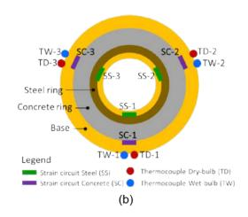
Figure 1: Experimental setup showing (a) photograph of the station with its parts labelled, and (b) schematics of measurement positions and instrumentation arrangement. "MP" stands for Measurement Position.
