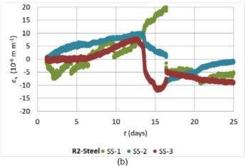
Figure 4: Graphs (a) and (b) show strain measured on the inner circumference of the steel ring in the hoop direction for rings R1 and R2 respectively while graph (c) shows strain measured on the outer circumference of the concrete ring in the hoop direction for ring R2. Time t = 0 corresponds to the casting of concrete and measurements started at  $t \approx 1$  day. Concrete ring R1 was made with medium strength concrete while concrete ring R2 was made with medium strength concrete made
