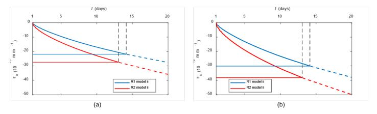
Figure 3: Time development of the strain in a) concrete ring,  $\varepsilon_c$ , and b) steel ring  $\varepsilon_s$ , determined by the numerical model (ii) for R1 and R2 concrete. The vertical black dashed lines denote the critical time,  $t_{cr}$ . The corresponding strain in the concrete,  $\varepsilon_c$ , and the steel,  $\varepsilon_s$ , rings are marked with the horizontal solid lines for the mixes R1 (blue line) and R2 (red line).
