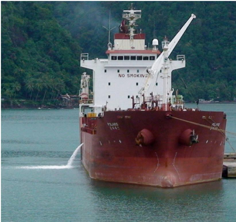
**Fig. 1: Ballast water discharge from a vessel in a port.**
