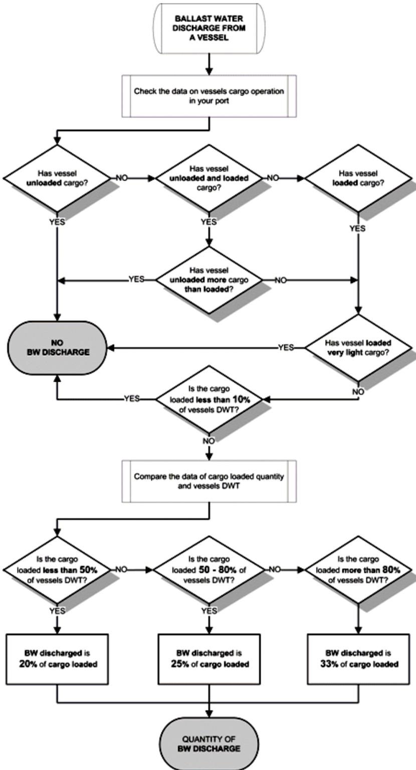
Fig. 3: Ballast Water Discharge Assessment (BWDA) model (David et al. 2012).
