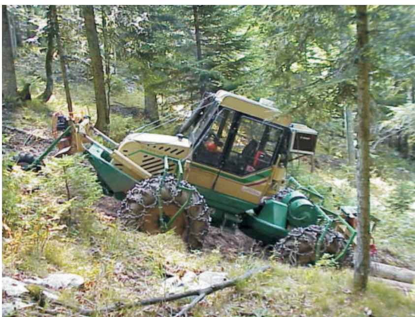
Fig. 2: WOODY 110 cable skidder during test at the stopping point
