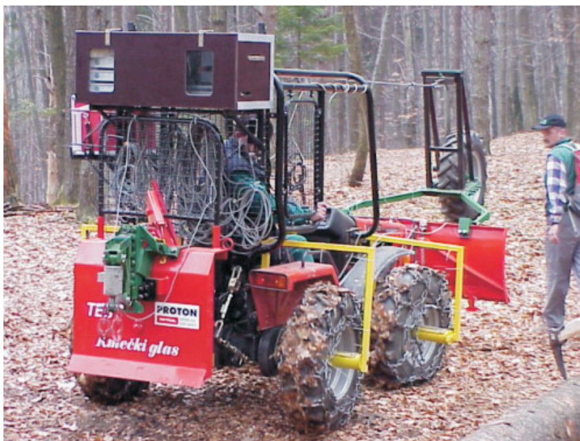
Fig. 1: AGT 835 with basic forestry equipment and measuring instruments during the test
