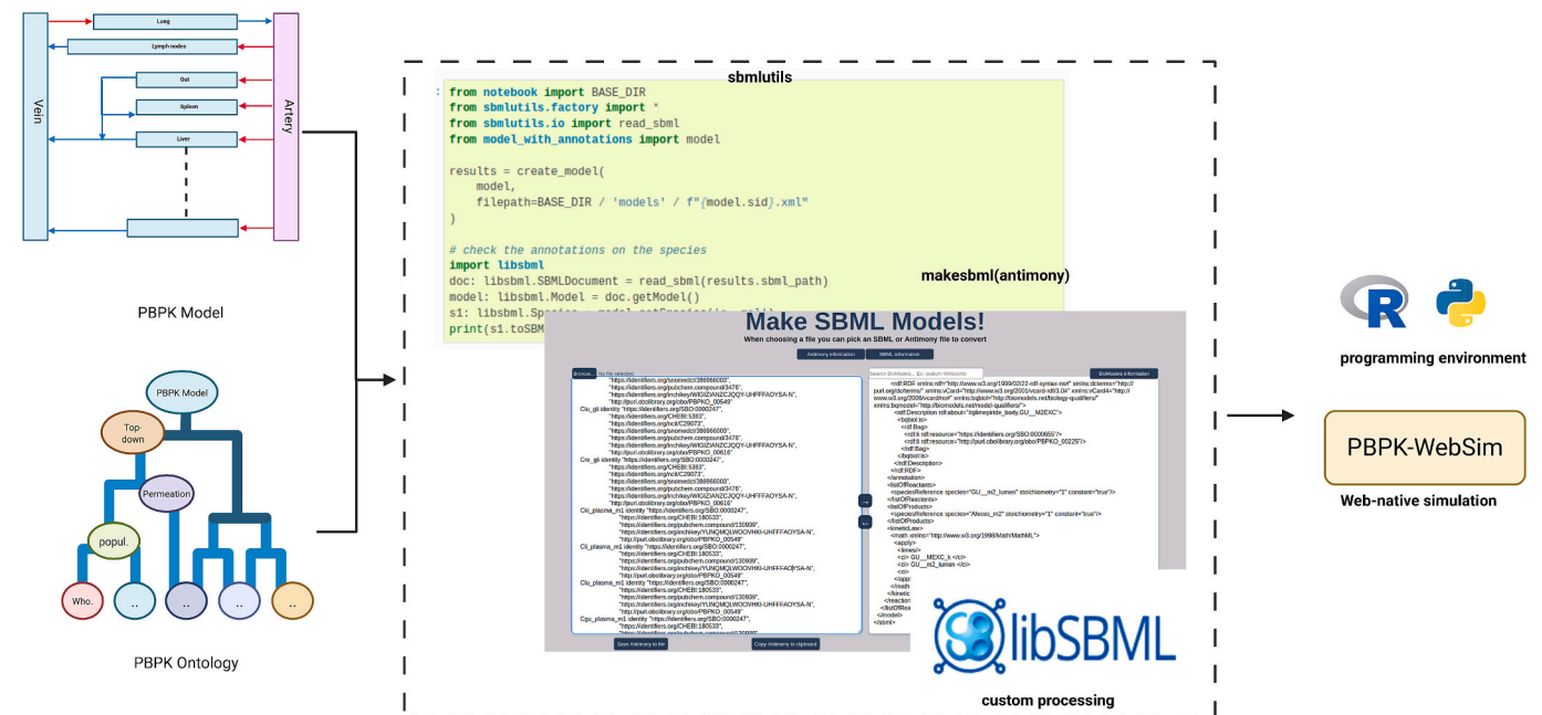
Fig. 4. Ontology-guided PBPK modelling pipeline. Three complementary approaches are used to annotate PBPK models in SBML format: (i) model construction and annotation using sbmlutils, (ii) Antimony-to-SBML conversion followed by annotation, and (iii) custom SBML processing using libSBML. The resulting annotated SBML models can be used for simulation and analysis in R, Python, or native web-based simulation platforms such as PBPK-WebSim [26].
