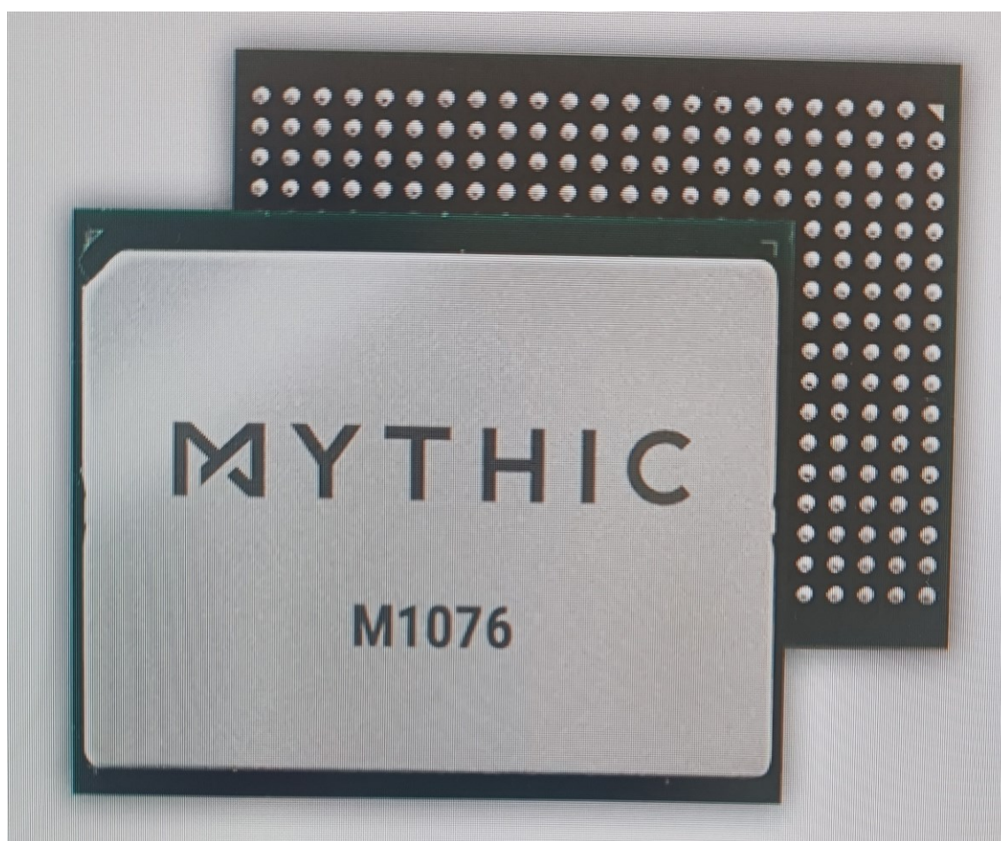
Figure 5: Analog mother processor that delivers analog computing for artificial intelligence that is comparable to a digital device with precision and power, MYTHIC, Austin, Texas, 2012, ( https://mythic.ai/ )
