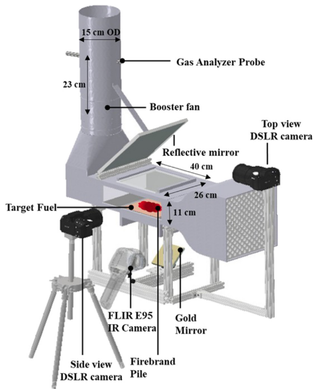
Fig. 1. A bench-scale wind tunnel setup used in this study drawn to scale. Source: Reproduced from Ref. [21].
