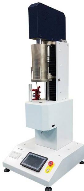
Slika 7: Automatic MFR / MVR Plastic Melt Flow Index Tester [15]
