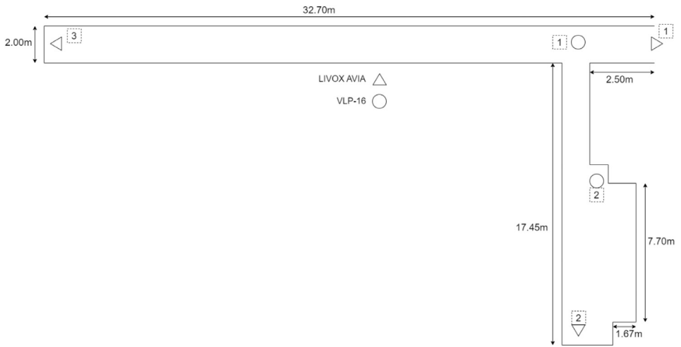
Fig. 5. Hallway with position of LiDAR system.
