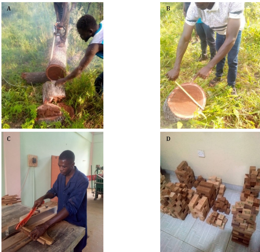
Fig. 1: Preparation of specimens for testing: A) felling of selected trees, B) measuring tree diameters, C) sawing specimens to the required sizes in accordance with selected standards, and D) prepared specimens ready for testing
