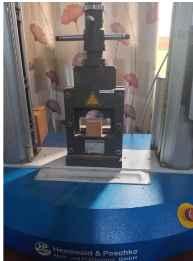
Fig. 3: Determination of shear strength parallel to the grain of P. kotschy specimens using an Instron universal testing machine
