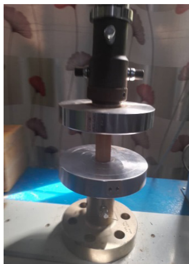
Fig. 2: Determination of compression strength parallel to the grain of P. kotschyi specimens using an Instron universal testing machine
