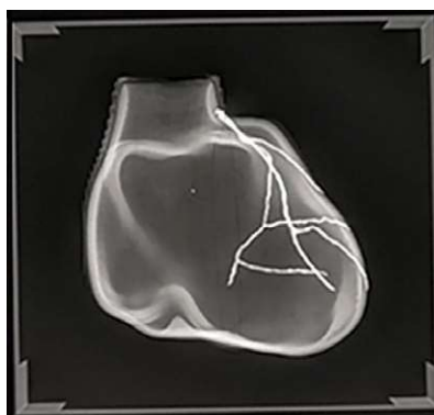
FIGURE 3. Radiograph of the heart model with vessels drawn by a mixture of UV gel and metallic powder.
