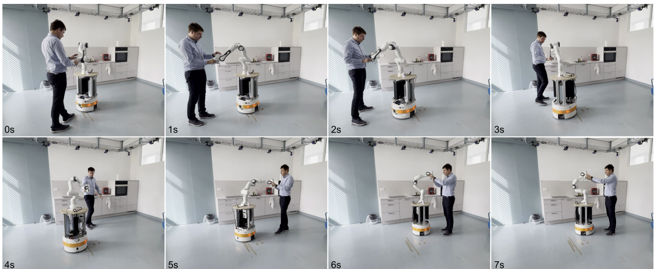
FIGURE 5. Sequence of kinesthetic guidance. As the operator physically moves the robot arm, the mobile base responds automatically by following the end-effector to maintain manipulability. This sequence corresponds to the experimental demonstration shown in Supplementary Multimedia 1.
