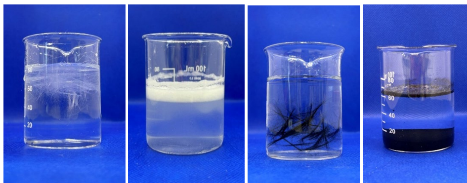
Figure 3: Sink-float method for (micro)fibrs (from left to right: f-PP, μf-PP, f-rPET, μf-rPET).
