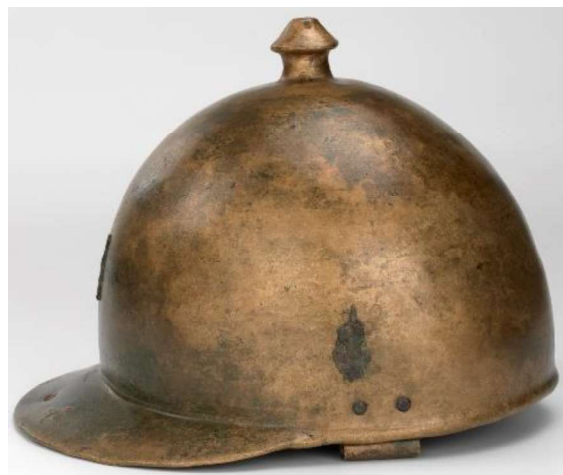
Fig. 4: Side of the C2 helmet (height 193 mm) from the River Ljubljanica. The helmet bowl is bronze (Cu with 10-11%). The cheek piece hinges are also bronze (Cu with c. 5% Sn) and the rivets that fasten them to the bowl are copper. The pure brass plume tubes (Cu with c. 14%, 22% and 23% Zn, respectively) were soldered to the sides and back of the bowl with a tin-lead alloy.
