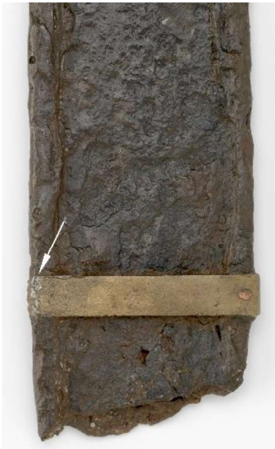
Fig. 7: Back of the A7 sword and scabbard (width 60 mm) from the River Ljubljanica; soldering (tin-lead alloy) at the brass crossband on the left and copper rivet on the right.
