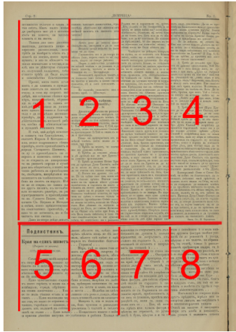
Figure 5: The same page from the Fig 4 additionally segmented vertically in columns which represent the order of the text in each horizontal area.
