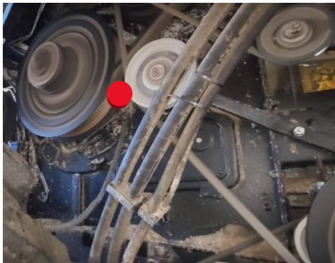
1 pav. Akselerometro matavimo vieta prie skriemulio L1 Fig. 1. Accelerometer measurement location at pulley L1
