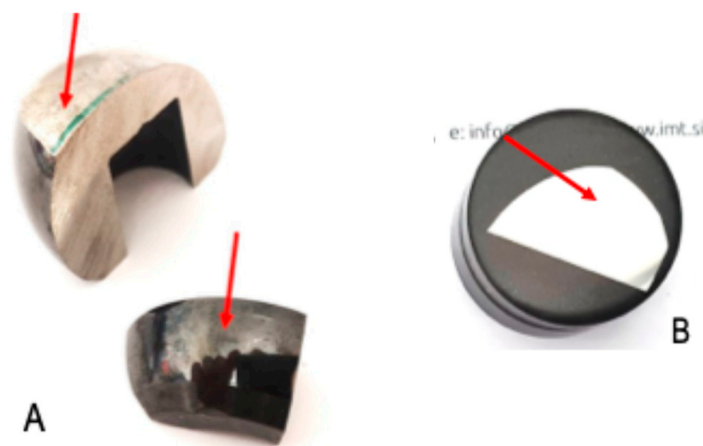
Figure 5. (A) Sample of retrieved Oxinium femoral head HV from the worn surface region, 383 HV, and from the diffusion layer, 1159 HV, as shown in Figure 6. Red arrow indicates the location of measurements. (B) Cross-section of metallographic sample of retrieved Oxinium femoral head used for hardness measurement.
