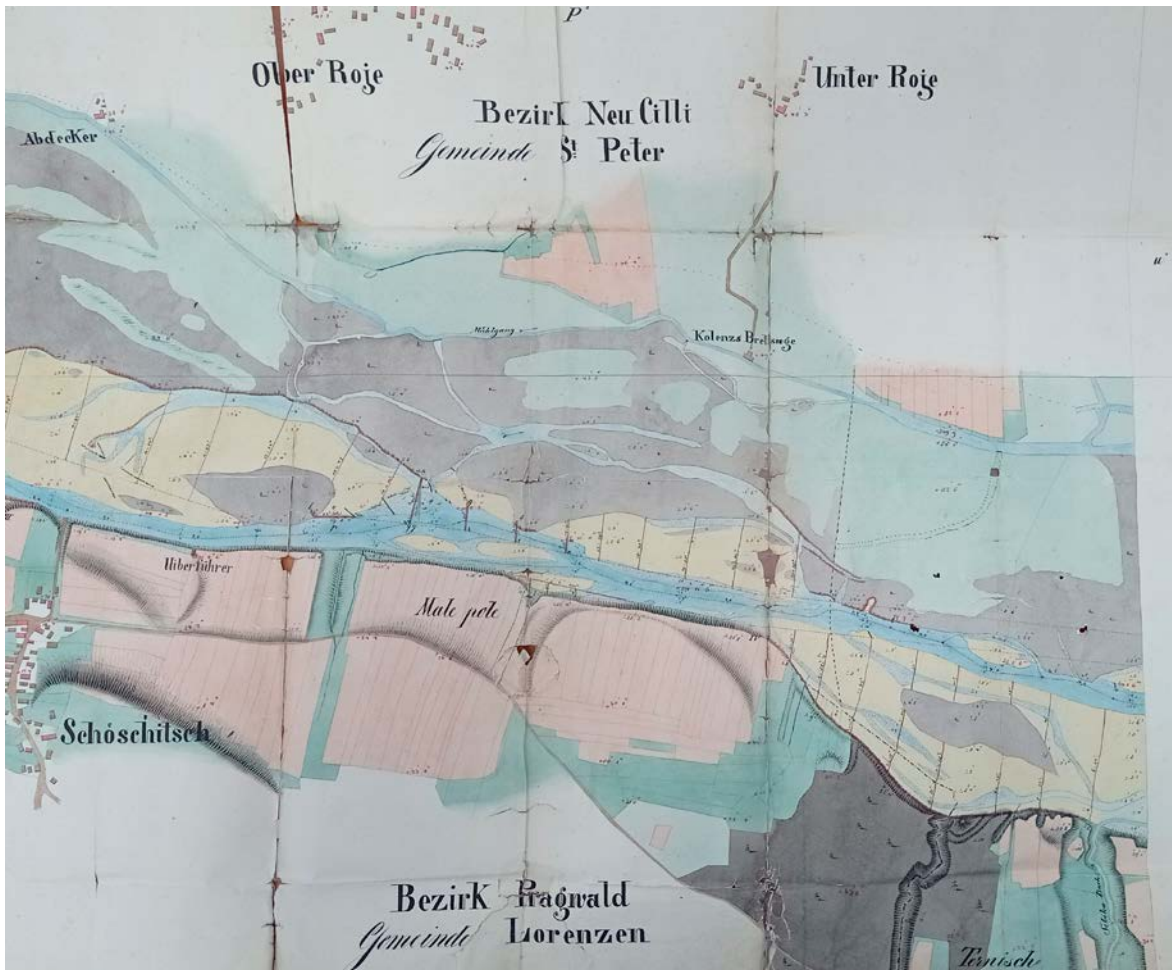
Fig. 1 Plan for reinforcing the banks of the Savinja in the district of Novo Celje, 1832.
