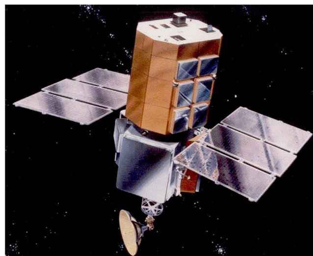
Fig. 1 | Image of the Solar Maximum Mission satellite, first repaired on orbit in 1984 by astronauts James van Hofton and George Nelson during a Space Shuttle servicing mission. The operation restored SMM's instruments and demonstrated complex rendezvous and hands-on servicing techniques that established confidence and methods later adopted by robotic and commercial on-orbit servicing efforts. Credit: NASA Marshall Space Flight Center (NASA-MSFC).
