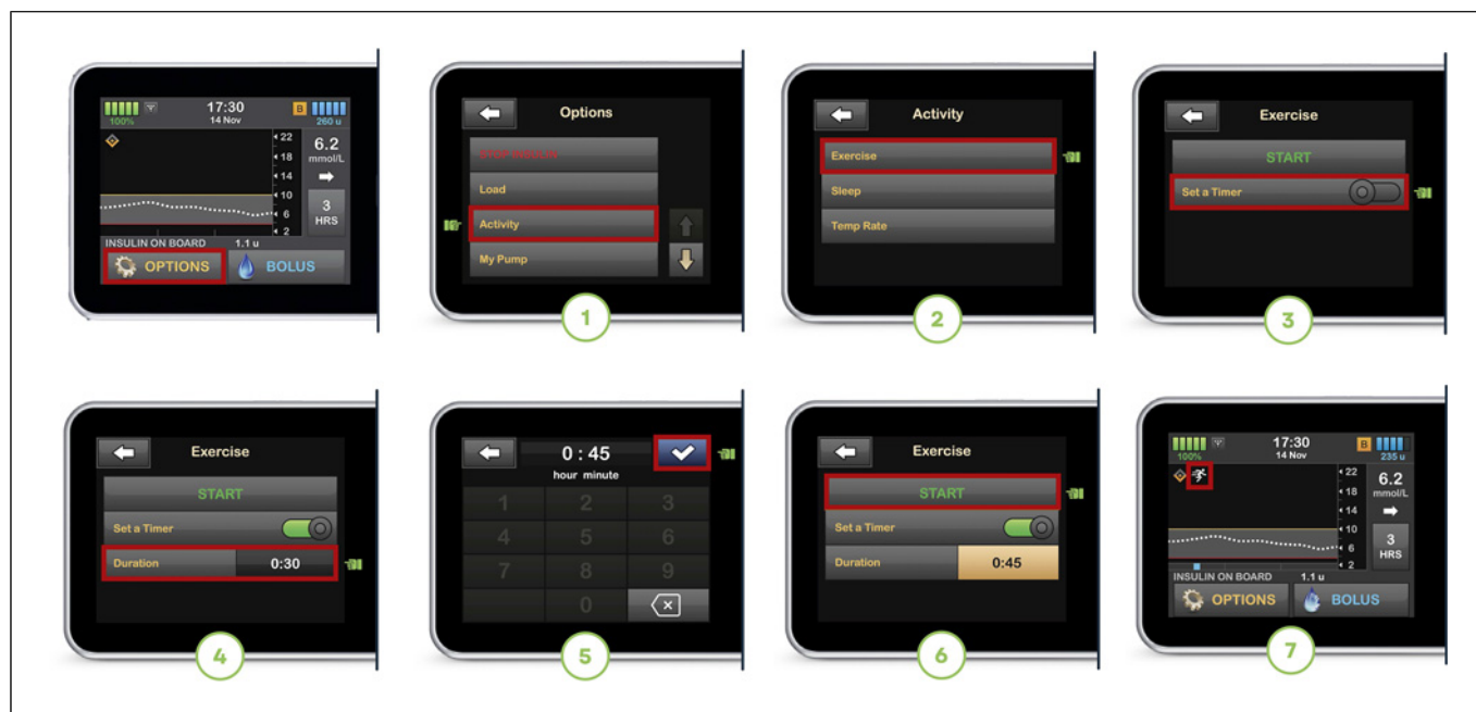
Fig. 11. Illustration of how to set the Exercise mode on the t:slim X2 Control-IQ system. See online supplementary ESM 1 for version of this figure with glucose concentrations in mg/dL. This figure is available as part of a downloadable slideset .
