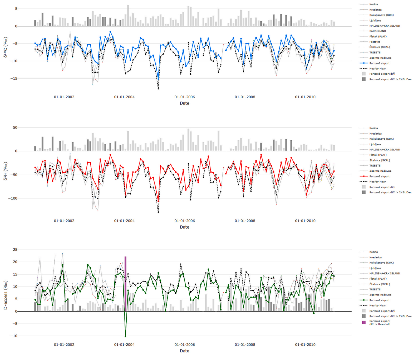
Fig. 5. Time series for the Portorož station (01.2001–12.2010) from the IsoQC app, displaying \delta^{18}\text{O} (top, blue), \delta^2\text{H} (middle, red), and d-excess (bottom, green) values. The solid-colored line represents data from the selected focal station, while the thick black dashed line indicates the mean values of nearby stations. Grey hairlines represent individual time series from neighboring stations within the defined search radius ( R = 110 km). Bars in the background highlight the difference of the elevation-corrected \delta_p and raw d-excess values between the nearby stations and the focal station, with purple bars marking D_{i,t} values exceeding user-defined thresholds and dark grey bars showing those difference values which are larger than two times the st. dev. of the data in the solving set for a particular month. Dataset . (For interpretation of the references to colour in this figure legend, the reader is referred to the web version of this article.) Source: SLONIP platform. For further information see Sect. 3.2
