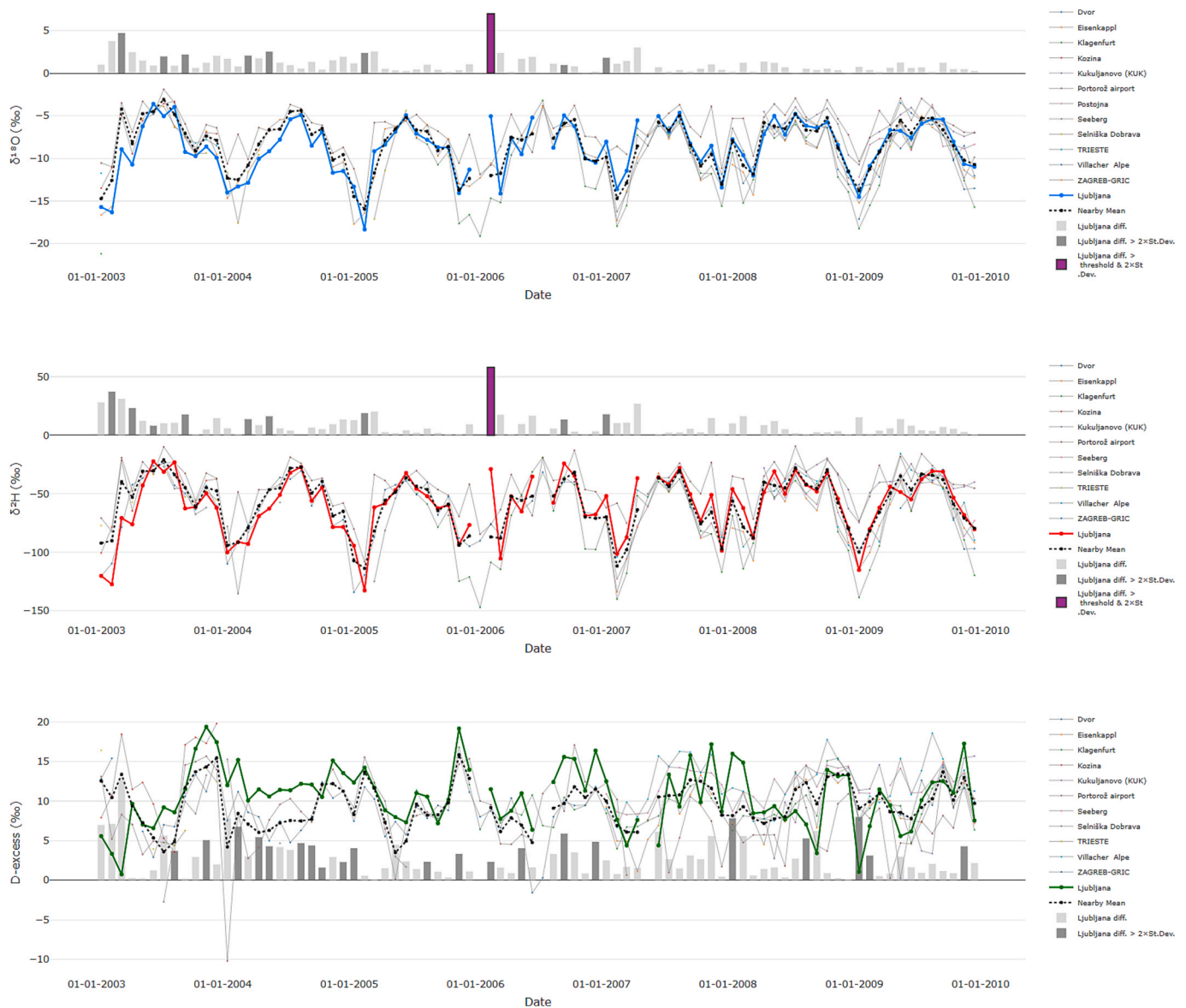
Fig. 6. Time series for the Ljubljana station (01.2003–12.2009) from the IsoQC app, displaying \delta^{18}\text{O} (top, blue), \delta^2\text{H} (middle, red), and d-excess (bottom, green) values. Dataset . (For interpretation of the references to colour in this figure legend, the reader is referred to the web version of this article.) Source: SLONIP platform. The search radius was set to 120 km to select the solving set. For a detailed description of the figure elements see the caption of Fig. 5
