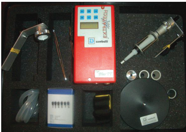
Figure 1: ZAMBELLI EGO PLUS TT personal sampler with associated sampling equipment
