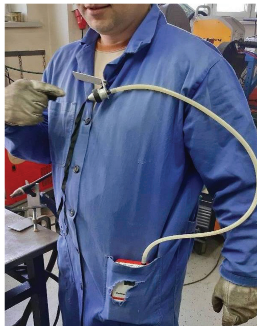
Figure 2: Position of the personal sampler in the operator's breathing zone
