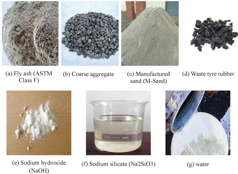
Figure ECF1: Materials used for the Geopolymer Rubberized Concrete
