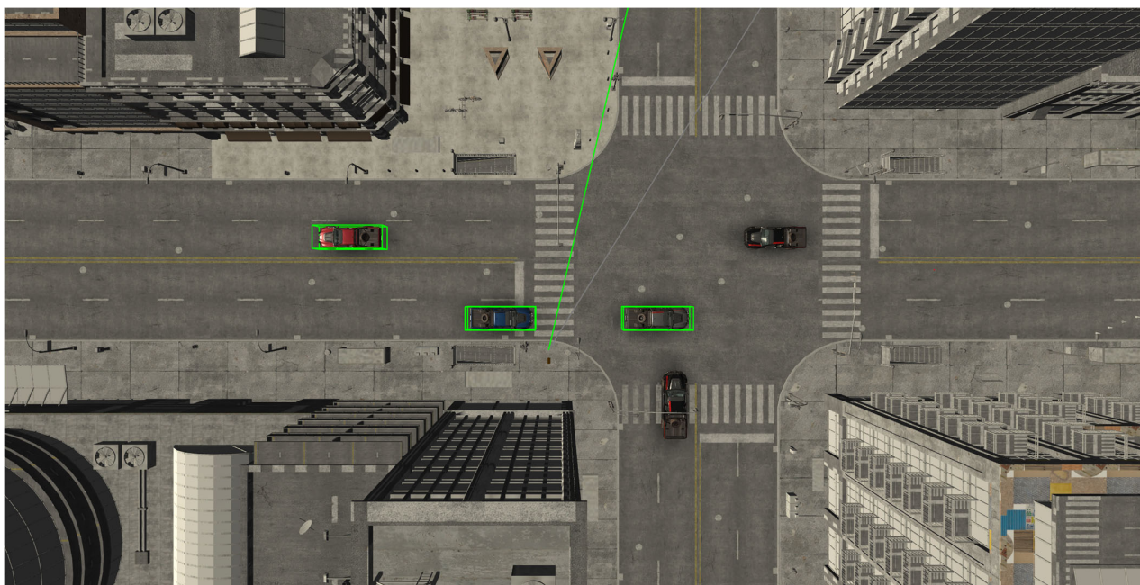
Figure 2. The view of the street with a pedestrian crossing and vehicles of different colours from above. The grey line shows the direction of the head in the VR, and the green line shows the direction of the gaze.
