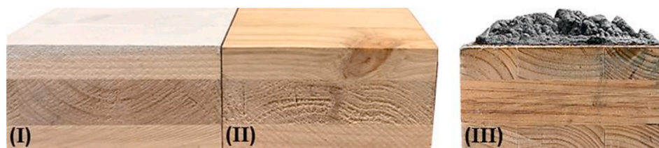
Fig. 1. Coatings applied on timber: (I) Opaque, (II) Transparent, (III) Transparent swelled.
