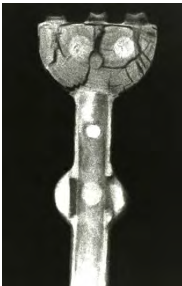
Figure B1.4 Neutron image of the upper part of the B1 dagger handle.
