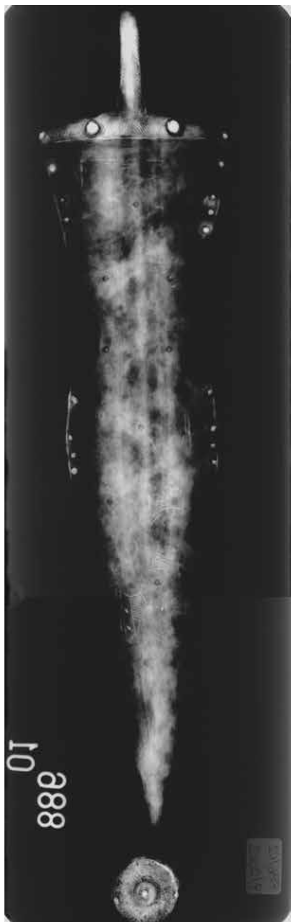
Figure B2.3 X-ray image (150 KV, 2.5 mA, 60 seconds) of the B2 dagger and sheath.
