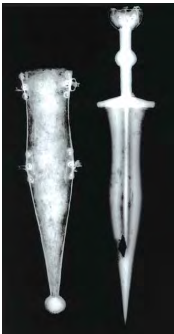
Figure B1.3 X-ray image (140 KV, 5 mA, 50 seconds) of the B1 dagger and sheath.
