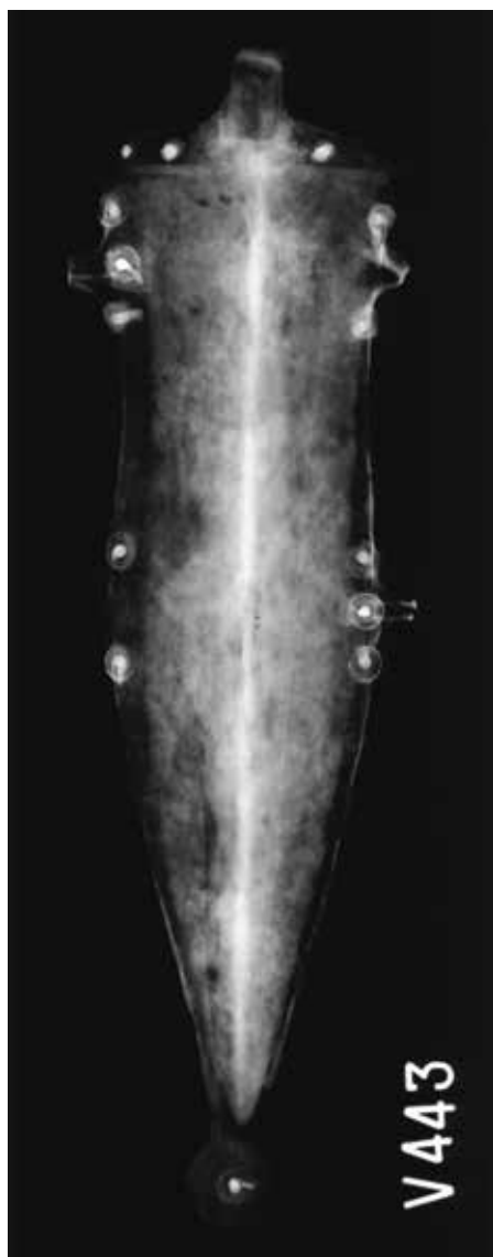
Figure B3.3 X-ray image (100 KV, 4 mA, 60 seconds) of the B3 dagger and sheath.
