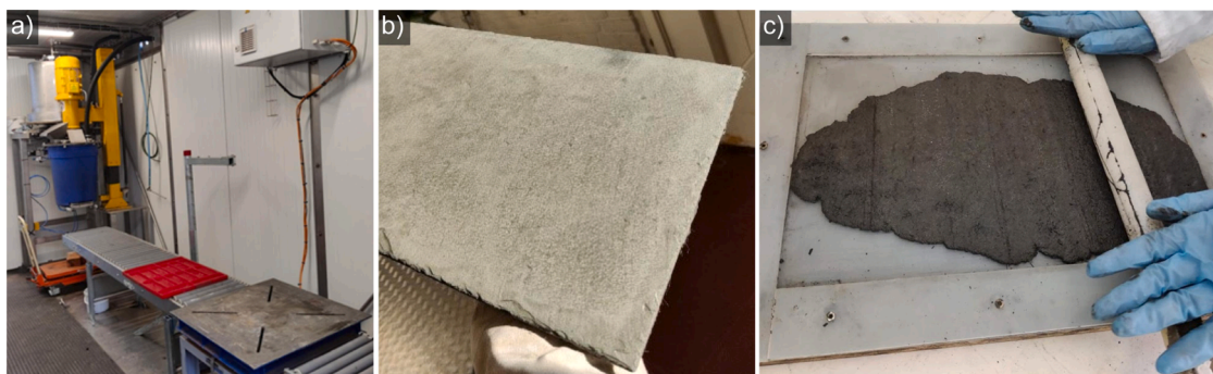
Fig. 6. Upscaling the pilot production: a) Production line used at SREMat KU Leuven, b) complete fibre layer and c) rolling on the cover layer in the mould.
