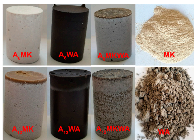
Figure 11. Photos of solid precursors and AAMs after 28 days of storage at room temperature.
