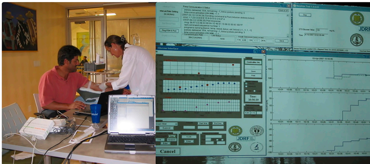
FIG. 2. The first model predictive control (MPC) study using the Artificial Pancreas System (APS) on April 10, 2007, Santa Barbara, CA. On the top right, it displays APS screens, including communication linking the Omnipod, Dexcom STS-7, main APS user interface (UI), and the real-time control/prediction algorithm. On the left, APS is running on a laptop connected via cables to the personal data manager (PDM) and the Dexcom receiver, next to our first participant.
