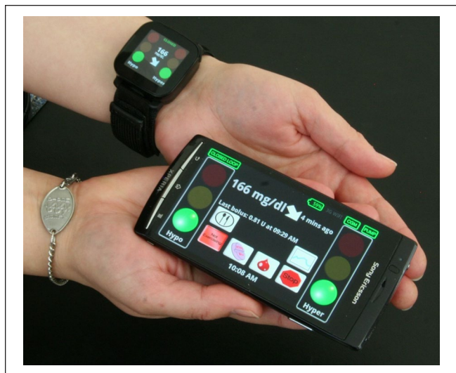
Figure 4. The Diabetes Assistant (DiAs), the first mobile glucose control platform.
