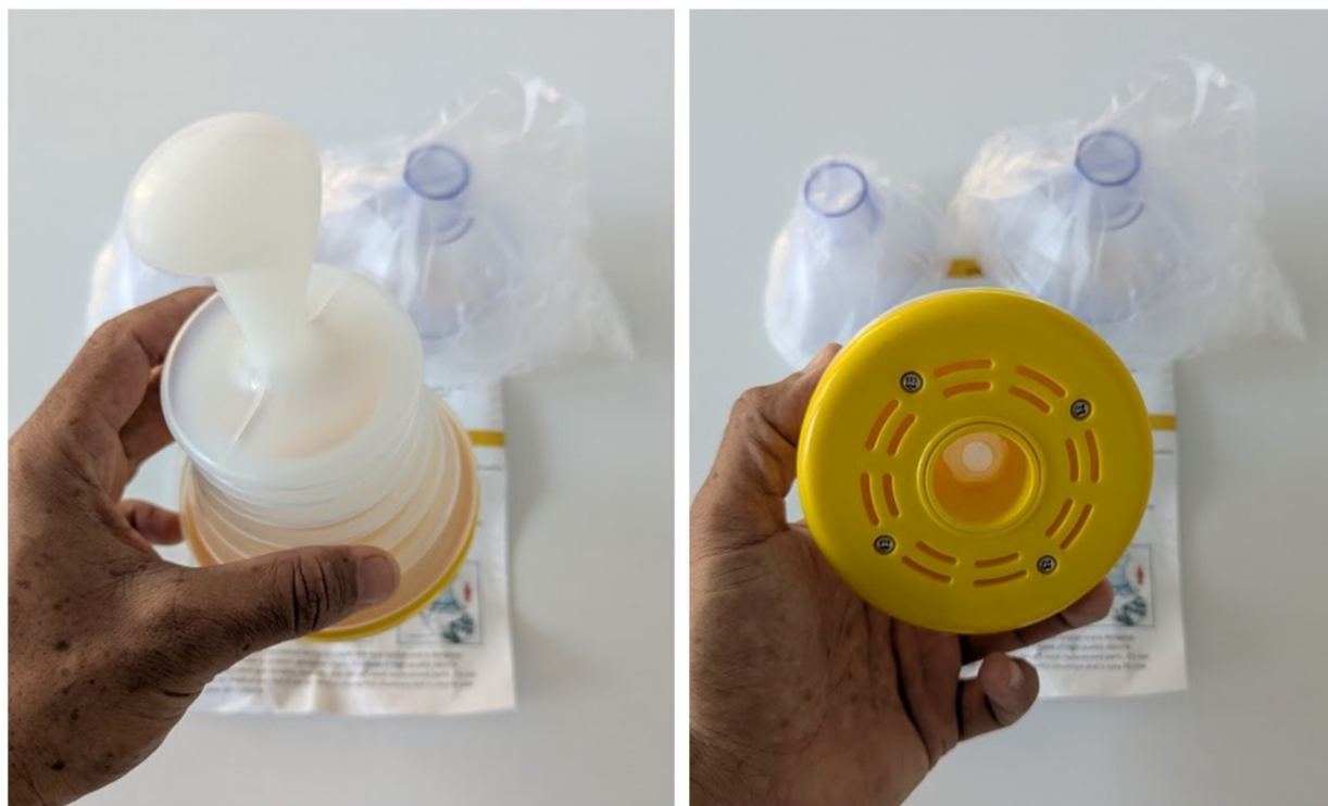
Fig. 1 – An example of a counterfeit anti-choking suction device without certification marks.
