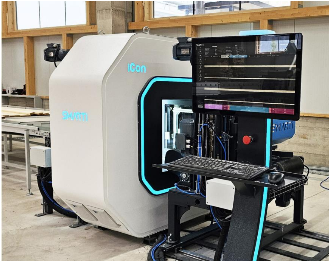
Figure 6: High-quality interface on the production line intended for four-sided 3D-scanning of boards for sorting in the production processes
