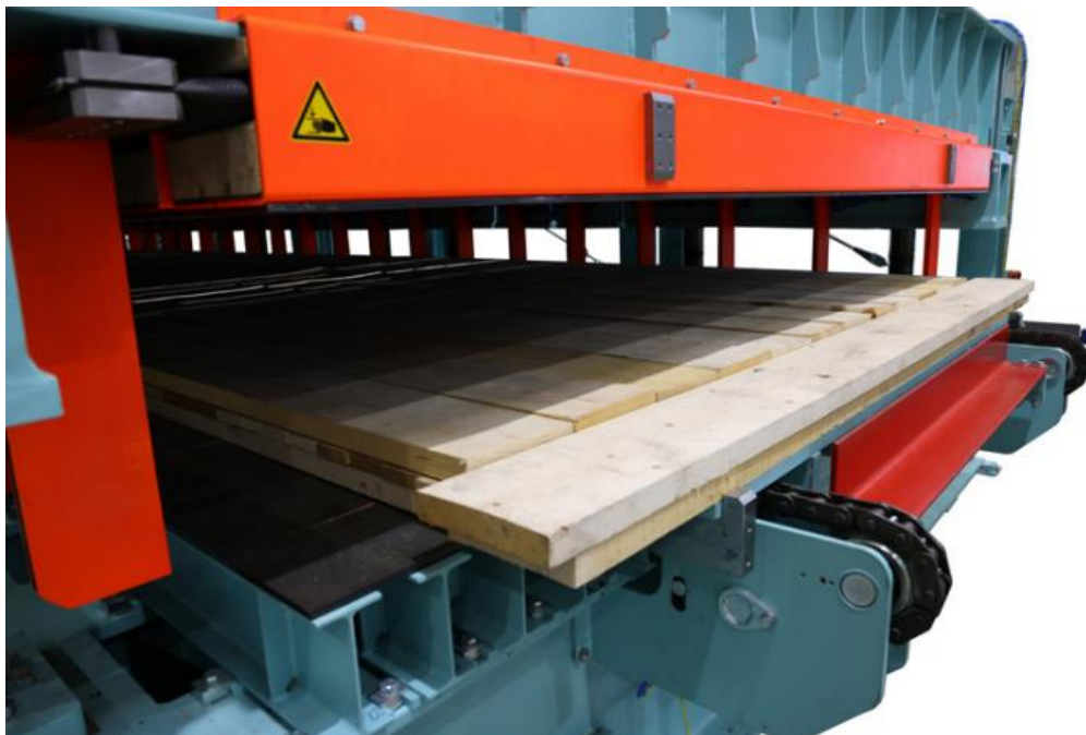
Figure 8: Optimised press for bonding CLT and GLT solid wood elements
