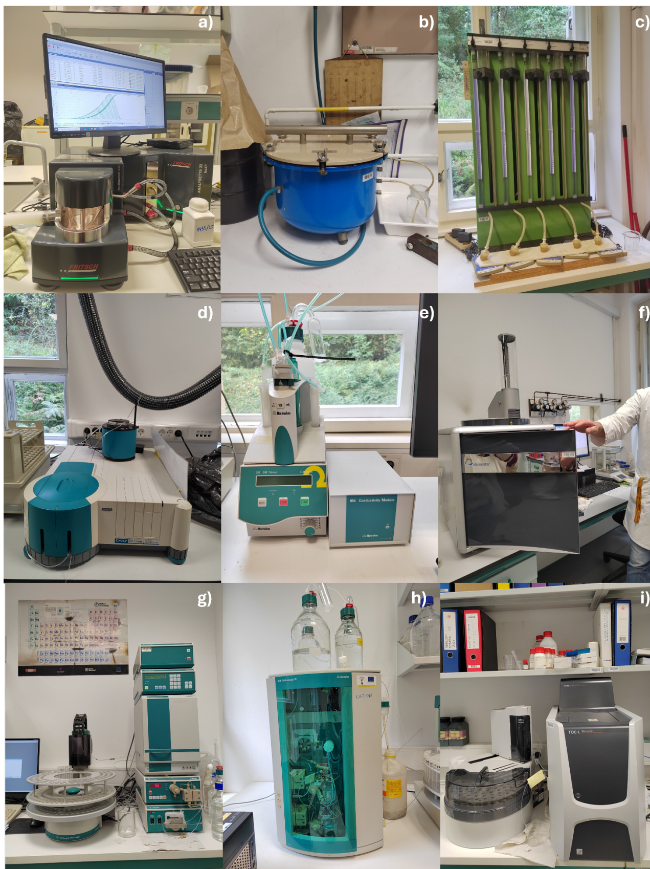
Figure 15: Soil physical property analyzers for soil particle size (a), soil water retention-PF curve (b); Soil chemical property analyzers: Calcimeter (c), UV-Visible Spectrometer (d), and Conductivity module (e); Solid sample analyzer for carbon, nitrogen, and sulfur (f); Liquid sample analyzers for Ions: Na, K, Mn, Ca, Mg, \text{NH}_4^+ , \text{NO}_3^- (g & h), as well as carbon and nitrogen analyzers (i).
