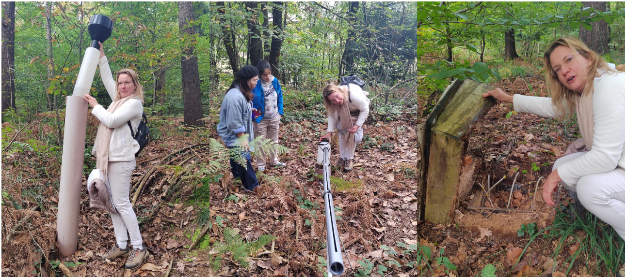
Figure 18: Devices for collecting precipitation (left), throughfall (middle) and soil water (right)
