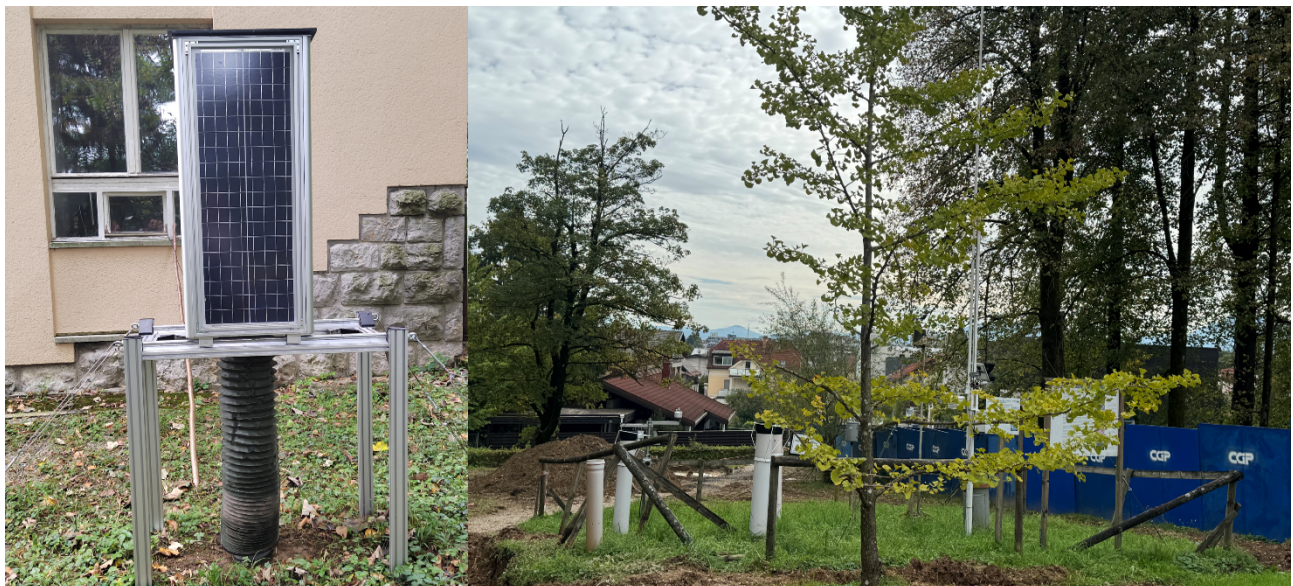
Figure 17: Automated soil respiration monitoring system (left) and meteorological site at urban forest research plot near the Slovenian Forestry Institute (right)
