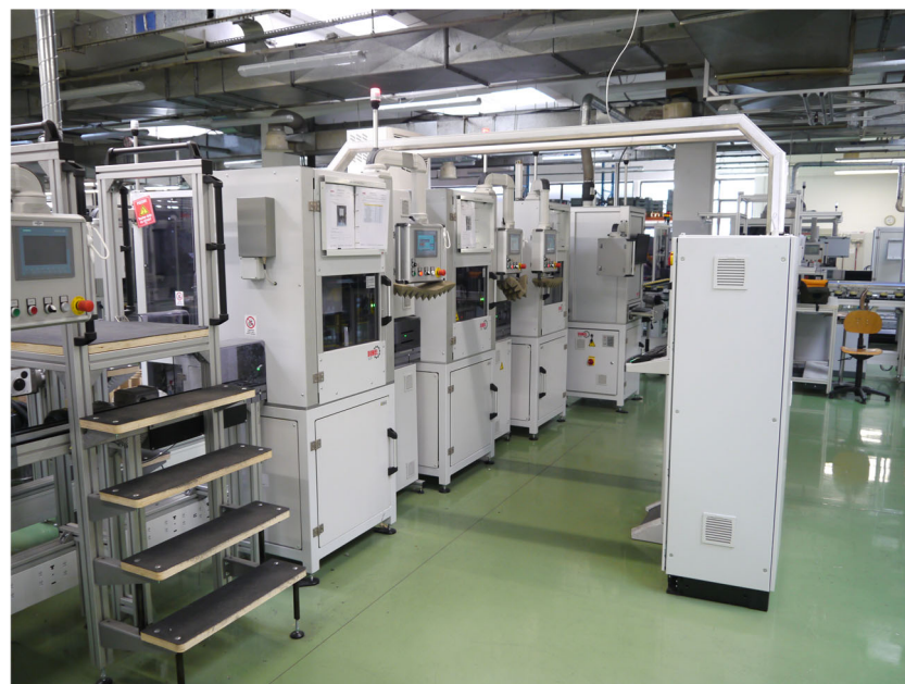
Figure 1. Typical End-of-Line quality inspection for electric motor production.
