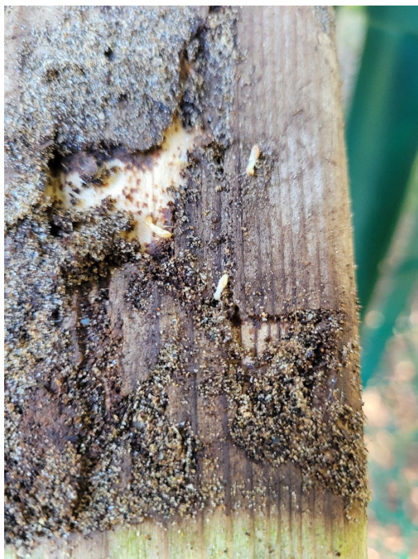
Fig. 4: Termite attack on an untreated red pine post installed in a boot (left) and failure of an untreated red pine post exposed in direct soil contact after 6 years (right)
