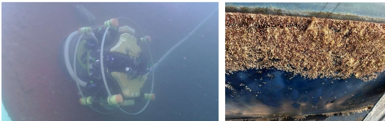
Figure 6. The ROV during an in-water hull cleaning operation in Portorož, Slovenia ( left ). The image shows the in situ deployment of the cavitation-based cleaning module and the real-time monitoring setup using the WiMo multiparametric probe. Demonstration of cleaning effectiveness using the developed cavitation-based hull-cleaning technology on a different vessel, shown out of the water for clarity ( right ). The image presents a section of the ship hull with an uncleared area covered by marine biofouling and an adjacent cleaned area below, where biofouling has been successfully removed, leaving the antifouling paint (dark blue) largely intact. The same cavitation-based cleaning principle was applied in both cases.
