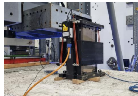
Figure 12. Placement of the vertical shaker on the girder.
