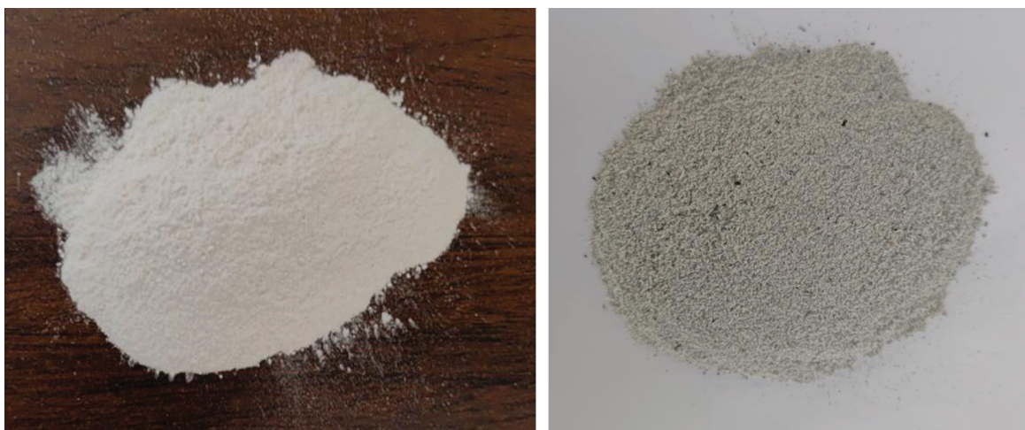
Figure 1: Steatite powder and micronized biomass silica
