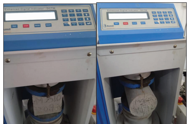
Figure 3: Testing of compressive strength and split tensile strength
