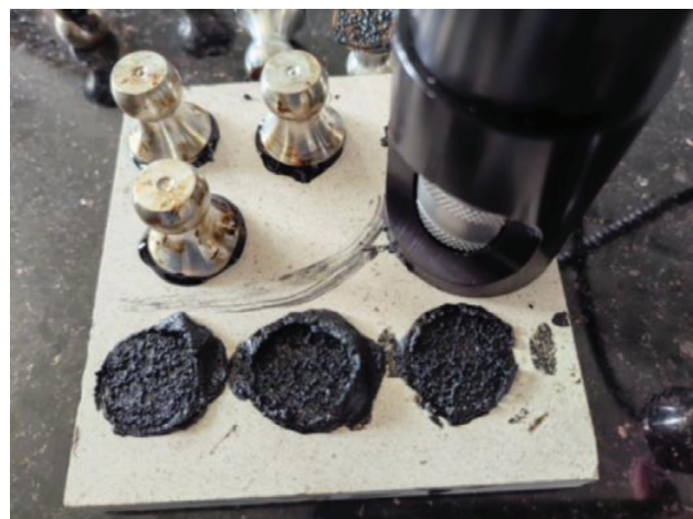
Figure 11: Failure morphology of the pull-off interface in the BBS test
