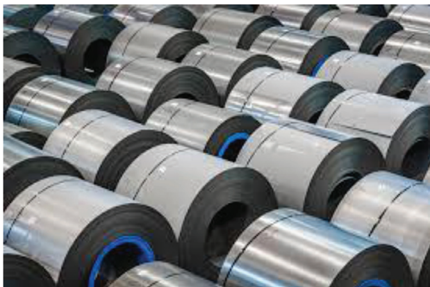
Figure 1: Coils of the fully-finished, non-oriented electrical steel (SIWATT brand of SIJ Acroni d.o.o., Jesenice, Slovenia) 1
