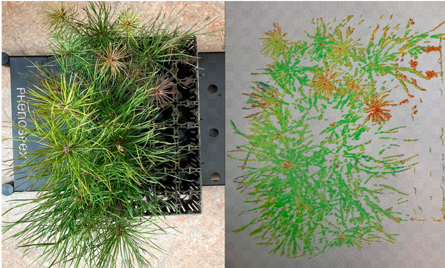
Figure 7.9 A multispectral 3-D scanner can rapidly collect large amounts of data that reveal early color changes caused by stress or infection in seedlings. Software translates the data to indices (e.g., NDVI) that can be used to evaluate plant condition. (Credit: Daniel Knapp, Linnaeus University.)
