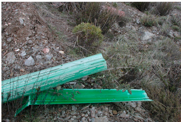
Figure 7.6 Plastic tree shelters photo-oxidize (degrade) and break into pieces, losing their ability to protect the seedlings or to support them if degradation is premature. (Credit: Juan A. Oliet.)
