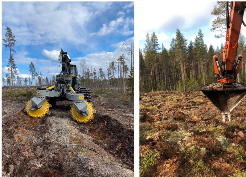
Figure 6.5 Mechanical site preparation using a disc trencher (left) and excavator and bucket (right) in SE Norway. (Credit: Jan Bjørnar Sankerud.)
