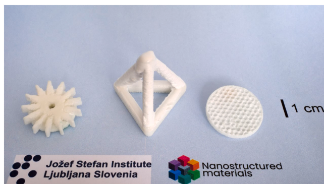
Fig. 12. Debinded and sintered parts after T3DP of 75 S3 feedstock.
