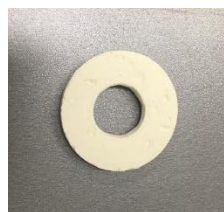
Figure 2. Picture of immobilised g\text{-C}_3\text{N}_4 catalyst on alumina substrate.
