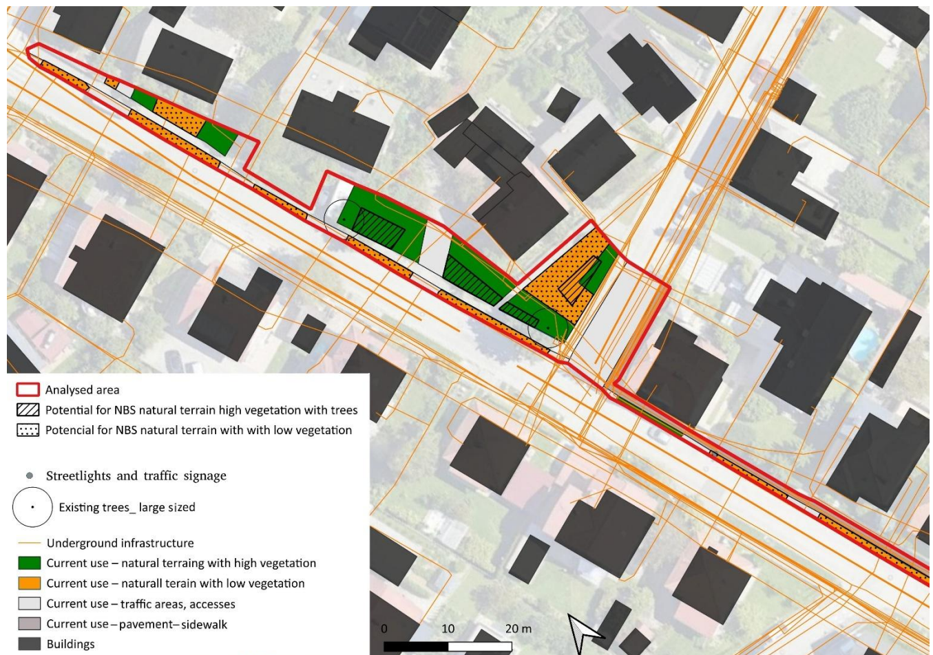
FIGURE 3. The results of the suitability assessment for implementing different NBS types on Street B indicate that only natural terrain high and Low Vegetation can be successfully implemented.
