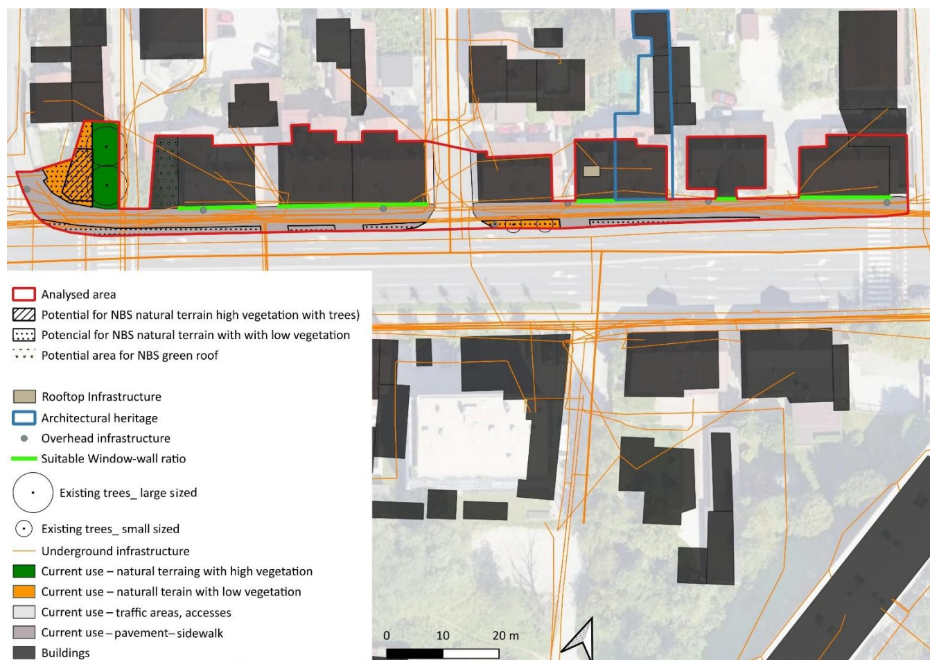
FIGURE 2. The results of the suitability assessment for implementing different types of NBS on Street A indicate that only natural terrain with High Vegetation and Low Vegetation can be successfully implemented.
