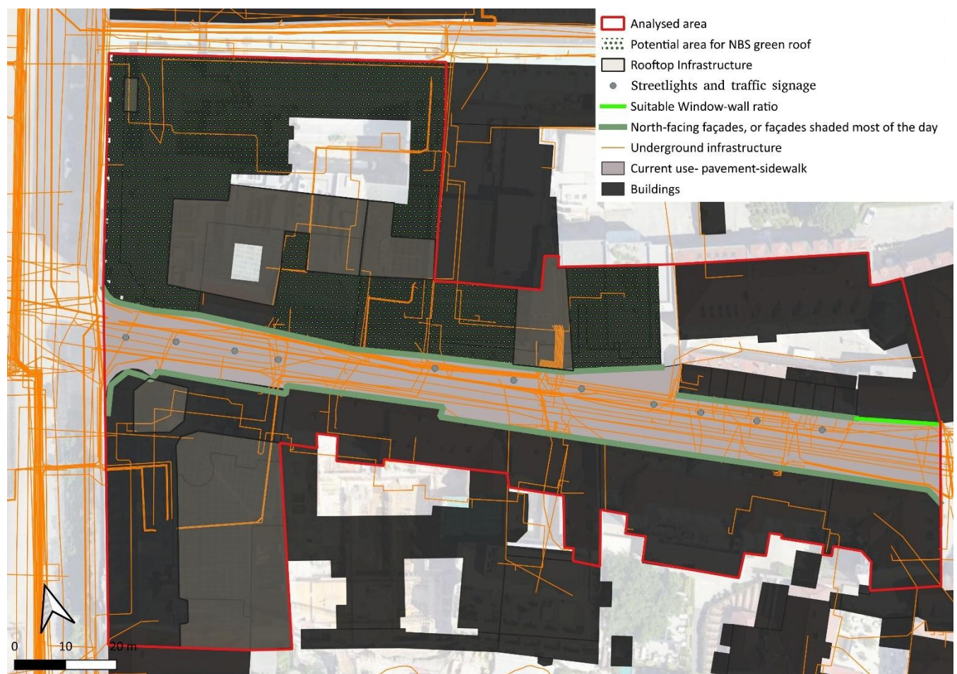
FIGURE 5. The results of the suitability assessment for implementing different NBS types on Street D indicate that only NBS green roof can be successfully implemented.
