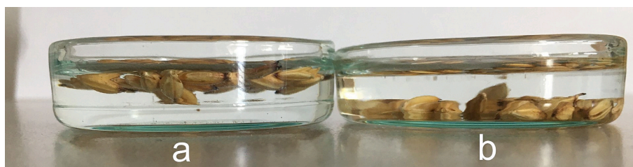
Fig. 6. Photo of: (a) as-received seeds with hulls that floated on the water and (b) seeds that sank in the water after treatment with oxygen plasma afterglow for 0.5 s.
