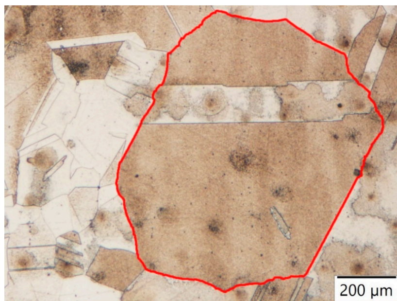
Figure 12. An exceptionally large austenitic crystal grain with a twin (grain boundary outlined with red).
