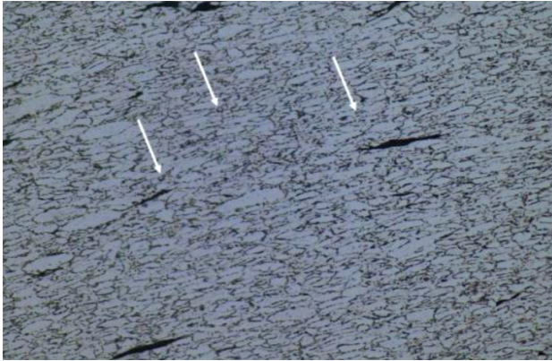
Figure 5: Metallographic microscopic image of the 0.5 w/% graphene/6061 Al composite at a strain rate of 2000 \text{ s}^{-1}
