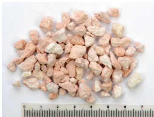
Slika 1. Laki agregat-Termit Figure 1. Lightweight aggregate-Termit
