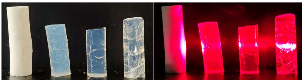
Figure. Silica monoliths at ambient light (left) and illuminated by laser light (right), showing their transparency.
