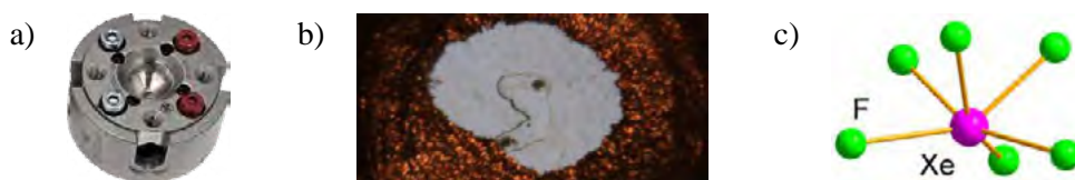
Figure 1. a) SS-DAC. b) Laser-heated sample in DAC. c) Structure of XeF 6 at 35 GPa with C 3v -like geometry.
